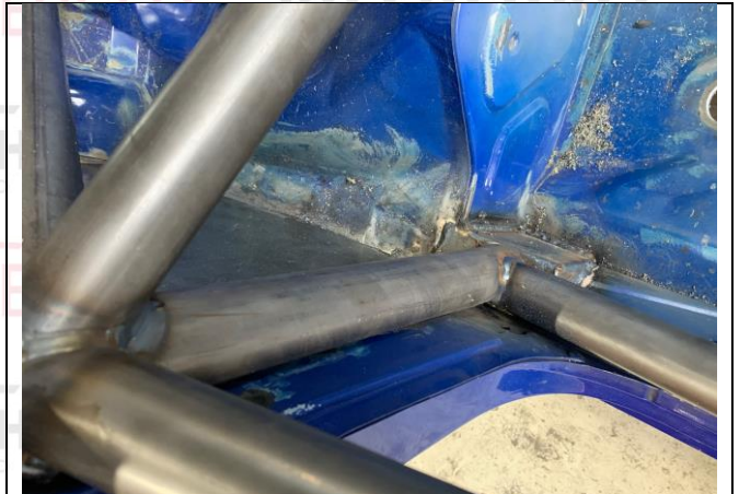
PHOTO 4 MAIN ROLLBAR TO FLOOR ATTACHMENT
