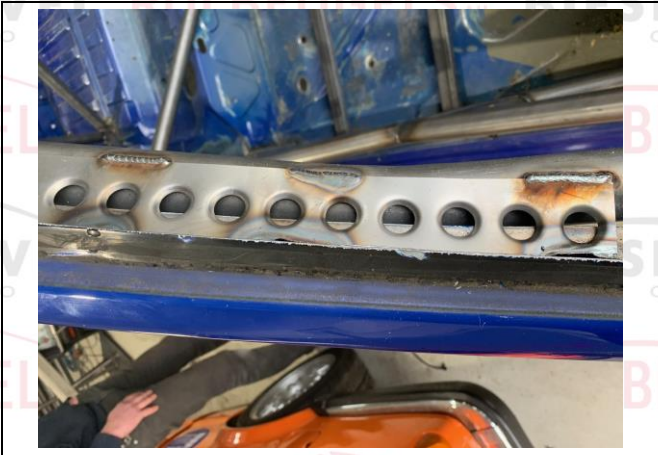
PHOTO 7 FRONT ROLLBAR TO "A" PILLAR ATTACHMENT
