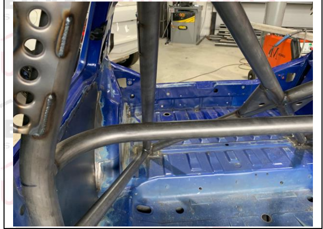
PHOTO 13 SHOULDER HARNESS ATTACHMENT - CO DRIVER
