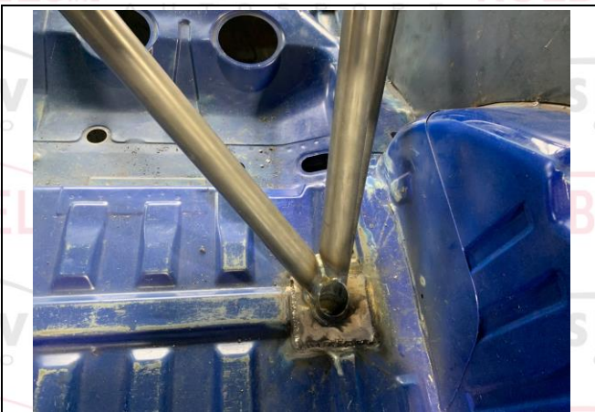
PHOTO 5 REAR BACKSTAY TO BODYSHELL ATTACHMENT
