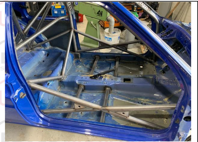
PHOTO 11 ANTI-INTRUSION DOORBAR – CO-DRIVER
